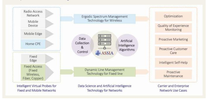
Fixed Line — Dynamic Line Management technology gathers data from fixed wireless, fiber, and copper access networks and fixed-edge computing equipment.
